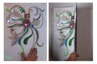
Figures 1 (left) and 2 (right). A paper computing project—an interactive "botanical design"—in which a microcontroller is used to control light and sound in response to a user's touch. A video can be found at the following URL: www.youtube.com/watch?v=-LyKmaz\_3ul
