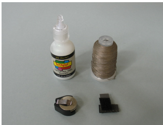
Figure 6.4: Power supply, switch, thread, and fabric paint.
