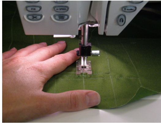
Figure A.6: Sewing the traces.
