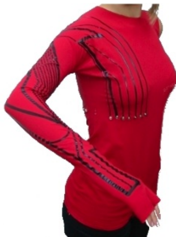
Figure 10.2: A shirt with embedded “piezo resistive” sensors.
