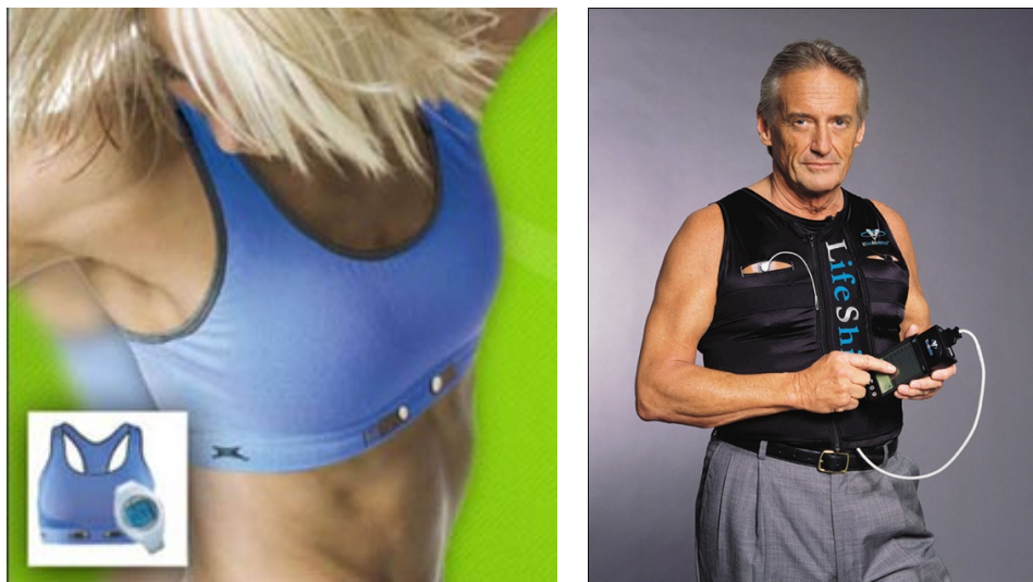
Figure 10.3: Commercial e-textiles: the heart-rate monitor bra by Numetrex and the LifeShirt by Vivometrics
