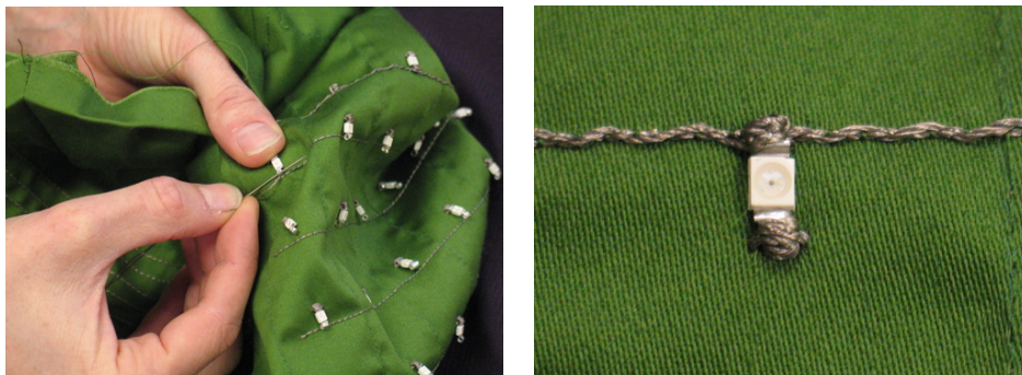
Figure A.10: Sewing in your LEDs.
