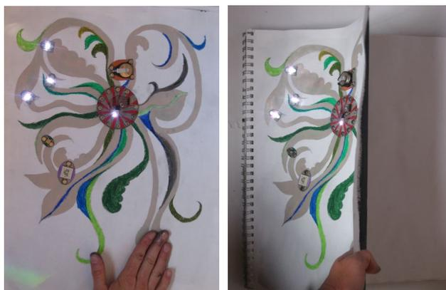
Figures 1 (left) and 2 (right). A paper computing project—an interactive “botanical design”—in which a microcontroller is used to control light and sound in response to a user’s touch. A video can be found at the following URL: [www.youtube.com/watch?v=LyKmaz\\_3uI](http://www.youtube.com/watch?v=LyKmaz_3uI)
