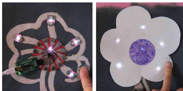
Figures 6 (left) and 7 (right). A paper computing project in which the circuitry is covered by 2 additional magnetic paper layers visible in Figure 7: a flower-shaped cutout and a circular purple cutout. Also visible in Figure 6 is the programming attachment.
