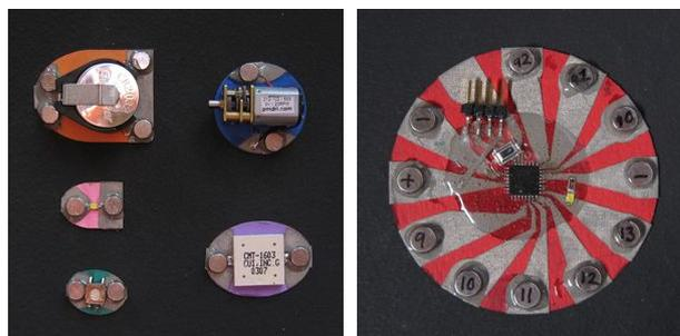
Figures 3 (left) and 4 (right). Components of our paper computing kit. Left: clockwise from upper left: a battery, motor, piezo speaker, switch, and LED. Right: a paper-based microcontroller; a paper Arduino.
